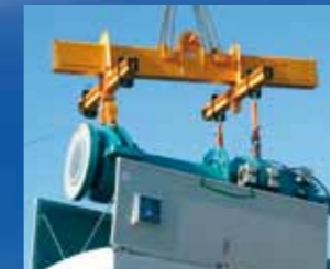
200 ton Lifting beam
